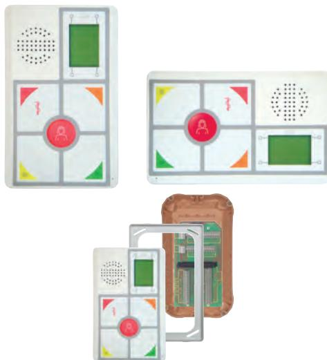
Room terminal with display for use as a decentralised call, operation and communication terminal with intercom facility in the patient's room, with integrated control and monitoring of all room functions. The terminal is connected to the ward bus and monitors all direct or via room bus connected devices.
