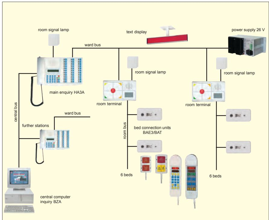
Each room terminal is a central switch and monitoring unit for all direct or via **room bus** connected devices in the room, at the patient beds and in the **sanitary facilities**.
